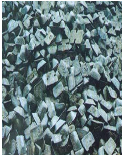
Gambar 3.21. Besi kasar ( pig iron )
