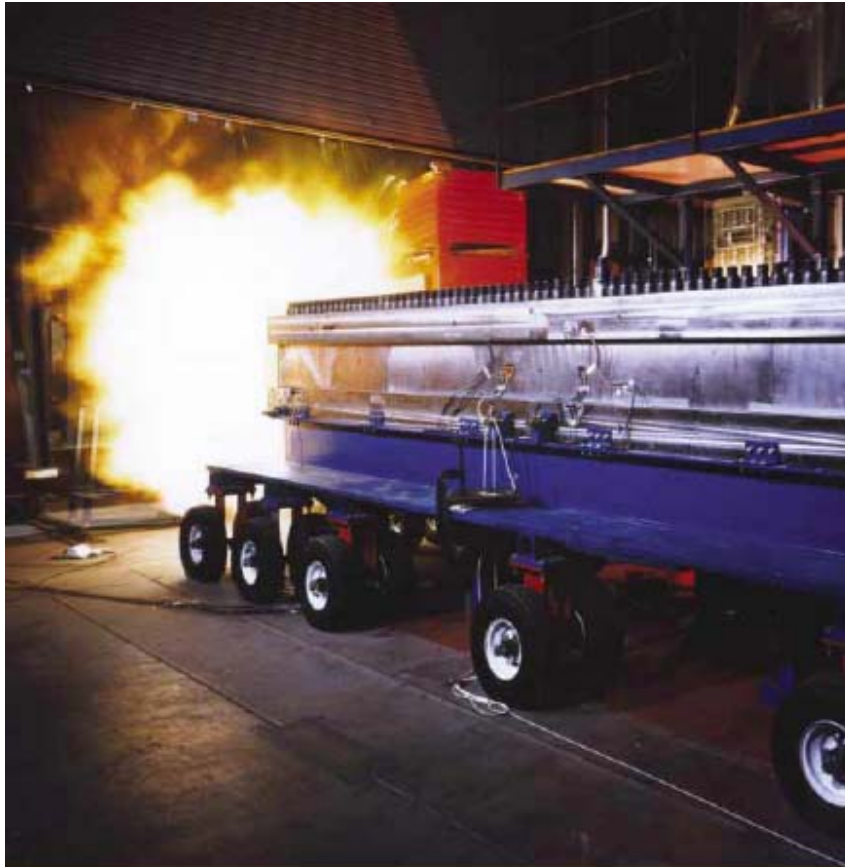
▲ A proposed method for launching future payloads into space is the use of rail guns, in which projectiles are accelerated by means of magnetic forces. This photo shows the firing of a projectile at a speed of over 3 km/s from an experimental rail gun at Sandia National Research Laboratories, Albuquerque, New Mexico. (Defense Threat Reduction Agency [DTRA])
