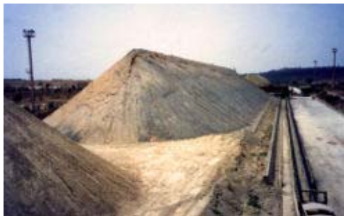
Gambar 20.70 Timbunan campuran bahan baku semen Portland
