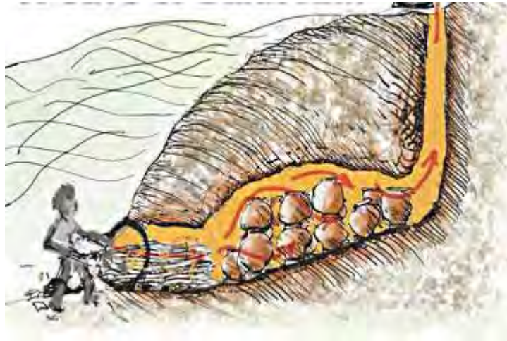
Gambar 8. Bank Kiln (Sumber: ceramicstudies.co.uk)
