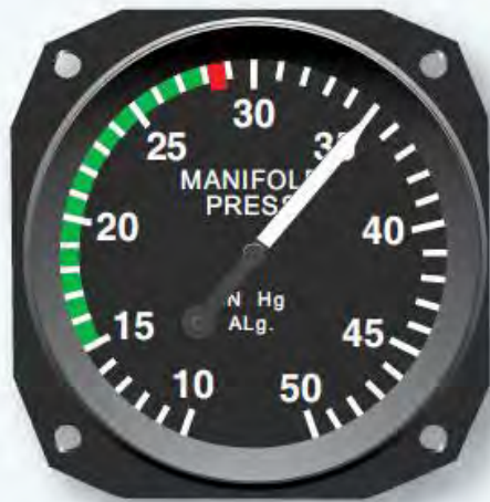
An analog manifold pressure indicator instrument dial calibrated in inches of mercury (left).
