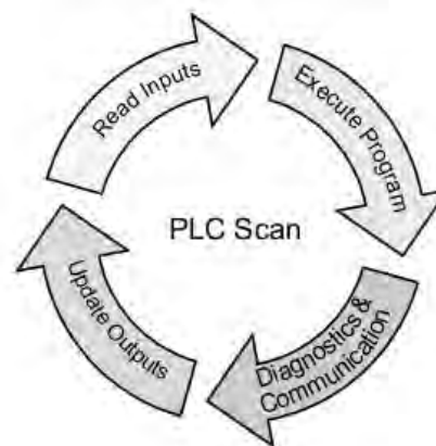
Gambar 4-21. Proses PLC scanning.
