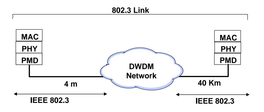
• The distances between switching equipment using the WAN PHY and the DWDM facility is commonly less than 2 Km
