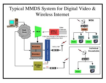
In a traditional wireless CATV system, each analog program received from a satellite downlink, local programming, or other source, would be modulated into the proper RF format to ensure reliable reception, combined with other channels to be broadcast to the same coverage area, amplified and transmitted to customers. Receiving antennas and set-top boxes installed at the customer's site would re-convert the RF signal into the format to be played on the TV or stereo.
