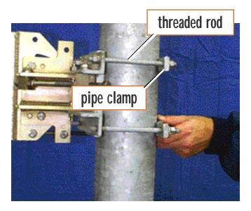
Make sure you have the right sized wrench as referenced above. Next locate the antenna base plate at the rear of the antenna and the two pipe clamps. The base plate and clamps are attached to the pipe mount via four threaded rods with associated nuts and lock washers (provided).
