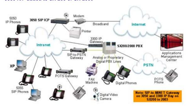
Where a Mitel Networks SX-200 or SX-2000 PBX is installed, the 3050 ICP can be used to cost-effectively add remote offices or single-user offices by adding a SIP-to-PSTN gateway (such as the Mediatrix 1204) connected to ONS lines on the PBX.
