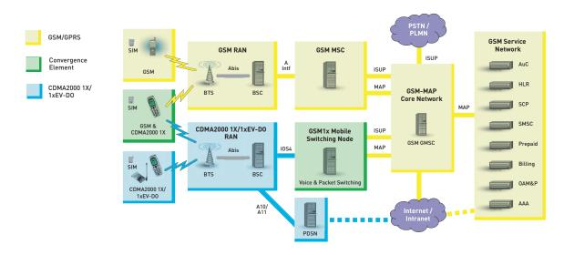
The GSM1x Global Gateway (GGG) enables a clear interface between a CDMA2000 network and a GSM-MAP network. The GGG ensures seamless transfer of GSM authentication and SMS parameters between the GSM-MAP network and GSM1x-compatible handset.
