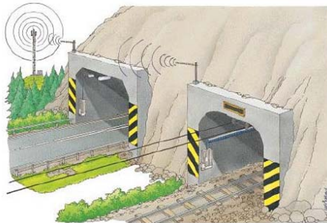
Figure 4 In-building coverage using repeaters (with the donor antennas visible on top of each tunnel entrance).
