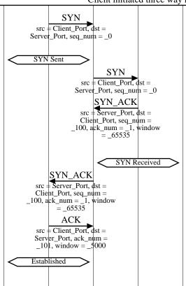
Client sets the SYN bit in the TCP header to request a TCP connection. The sequence number field is set to 0. Since the SYN bit is set, this sequence number is used as the initial sequence number
