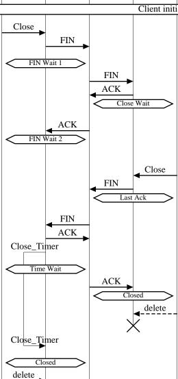
Client application wishes to release the TCP connection
