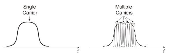
For example, instead of one signal carrying 72 Mbps of data, there are 48 separate carriers, each carrying about 1.5 Mbps of data (in the case of the Redline product).
