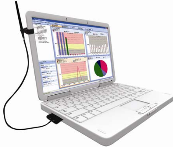
Figure 1 - Cognio's Spectrum Expert is the first spectrum analysis product design for WLAN applications. Source: Cognio, Inc.
