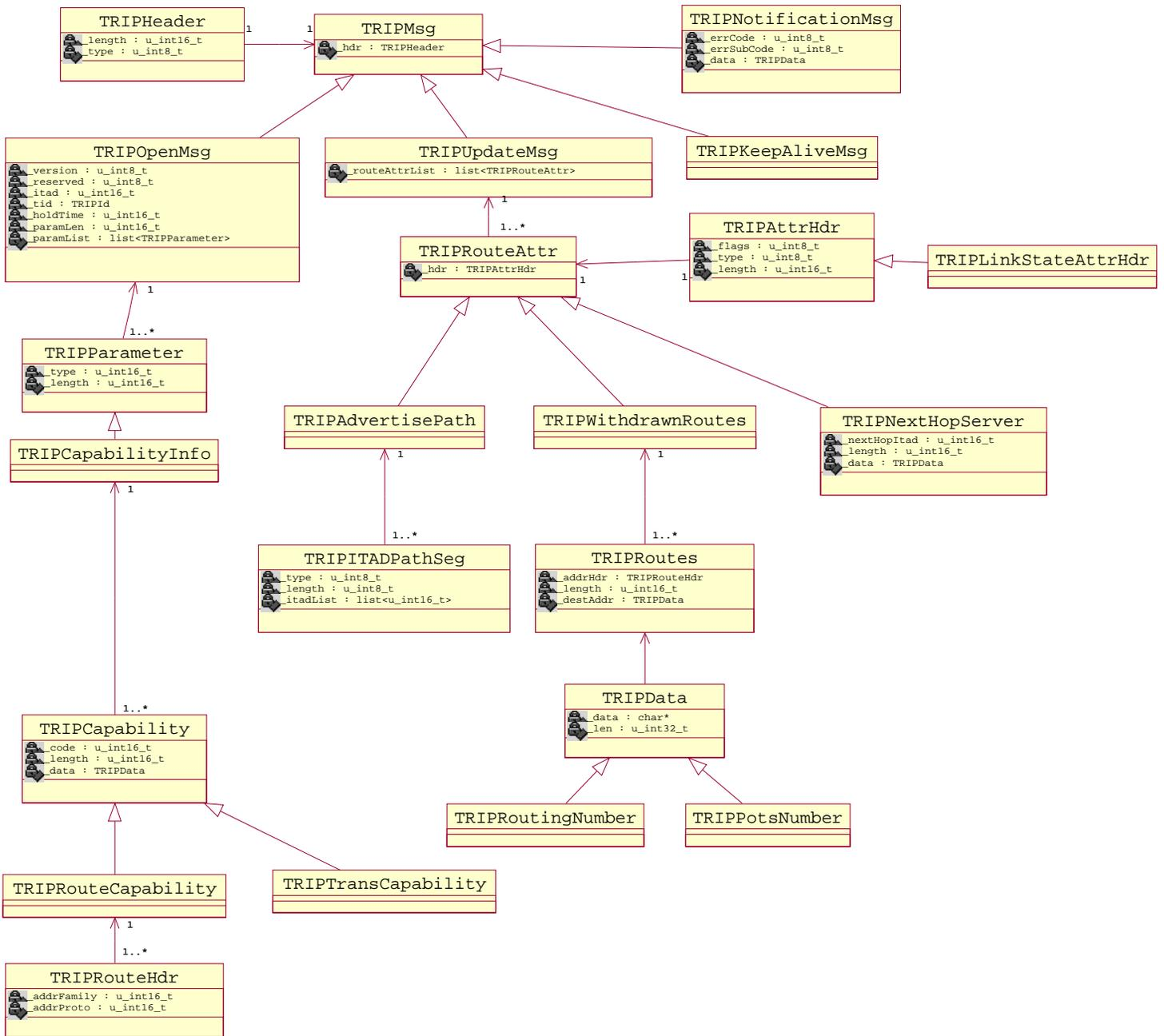
TRIP core - Implements the TRIP message format, encoding and decoding of TRIP messages.
