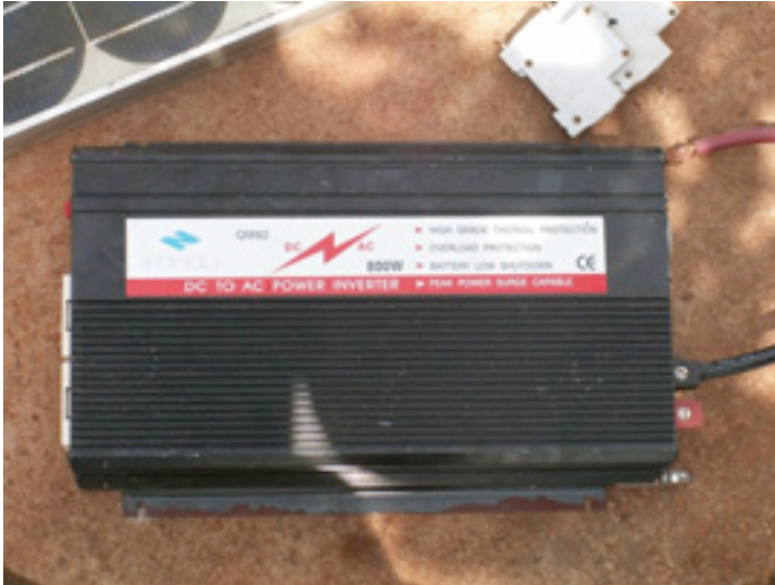
Figure 7.4: An 800 Watt DC/AC converter (power inverter)
