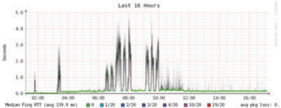
Figure 6.19: SmokePing can simultaneously display packet loss and latency spreads in a single graph.
