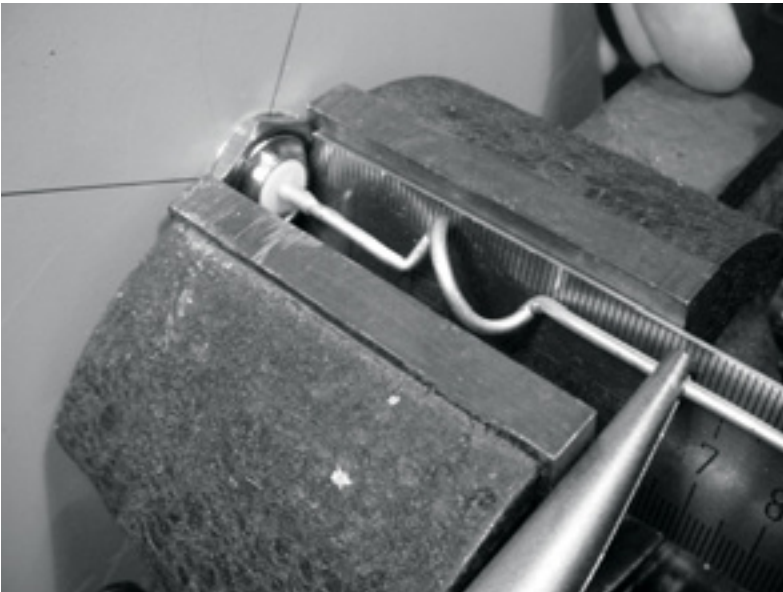
Figure 4.27: Stretching the coils. Be very gentle and try not to scrape the surface of the wire with the pliers.
