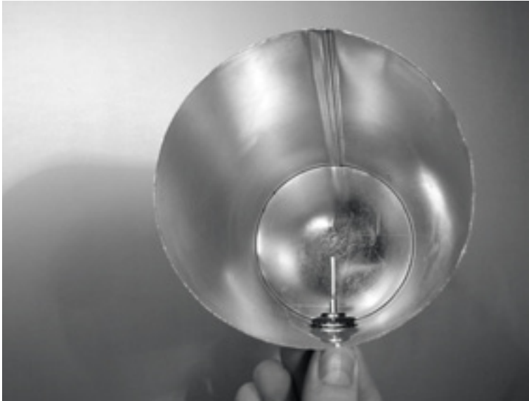
Figure 4.41: Your finished cantenna.
