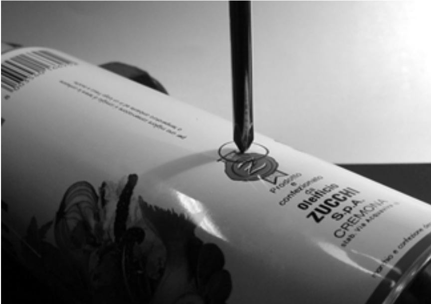
Figure 4.35: Mark the hole before drilling.
