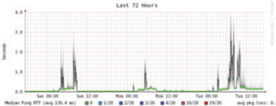
Figure 6.29: Zooming out to the week long view reveals a definite repetition of increased latency and packet loss in the early morning hours.
