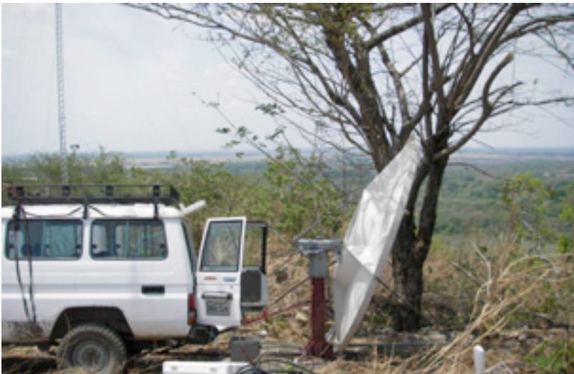
Figure 11.34: El Baúl antenna installation. Actual elevation was 1^\circ upward, since the antenna has an offset of 22.5^\circ .
