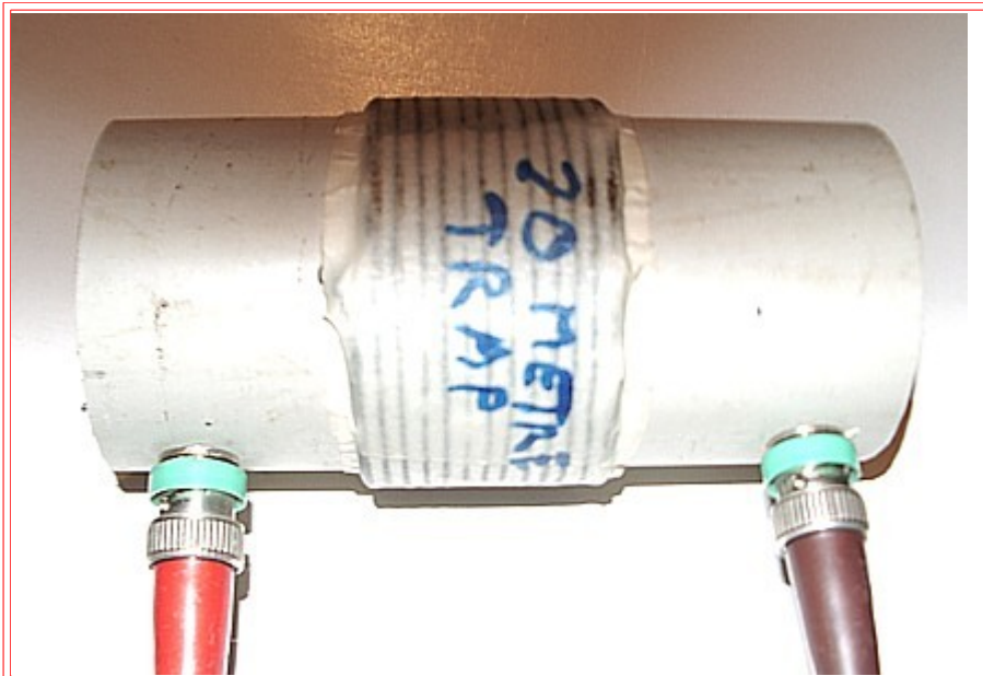
Photo 3 - 20 METRE TUNED TRAP
