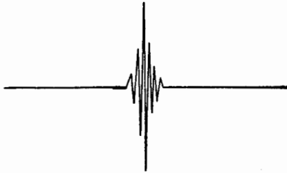
FIG. 1.3.—Modulated alternating voltage (short a-c pulse).
